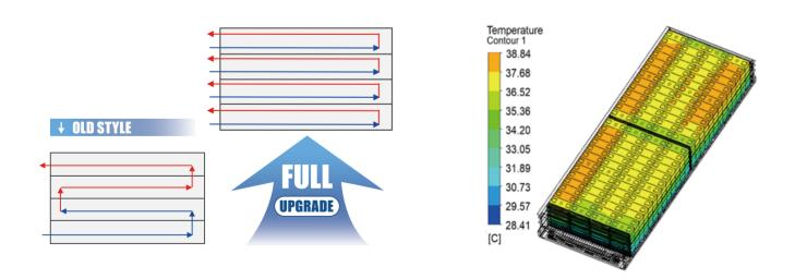
Compared with traditional serial flow channel, the flow resistance of parallel flow channel at the same flow rate is reduced by 85.5%. The maximum temperature difference between cells is kept under 2.78°C.
