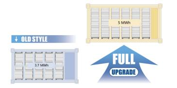
Nominal energy upgrades by 35% from 3.7MWh to 5MWh in a 20HQ container, due to internal space optimization, cell capacity upgrade and single-side maintenance. Battery capacity upgraded by 12% from 280Ah to 314Ah. Battery quantity increased by 20% from 4160 to 4992. Battery array increased by 20% from 10 to 12.
