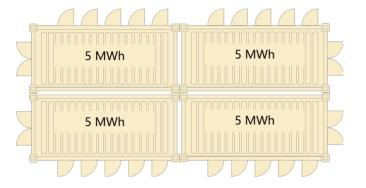
New model maximizes space utilization (improved by 26% from older version). With single-side maintenance design, containers can be installed back-to-back and shoulder-to-shoulder onsite.
