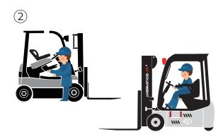
Lift up the driver seat and disconnect the battery.
