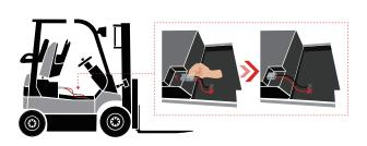
Plug in the EP Li-ion battery.
