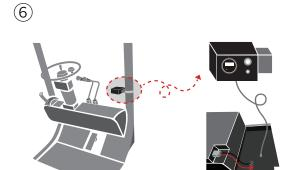
Attach the battery indicator to the cabin.
