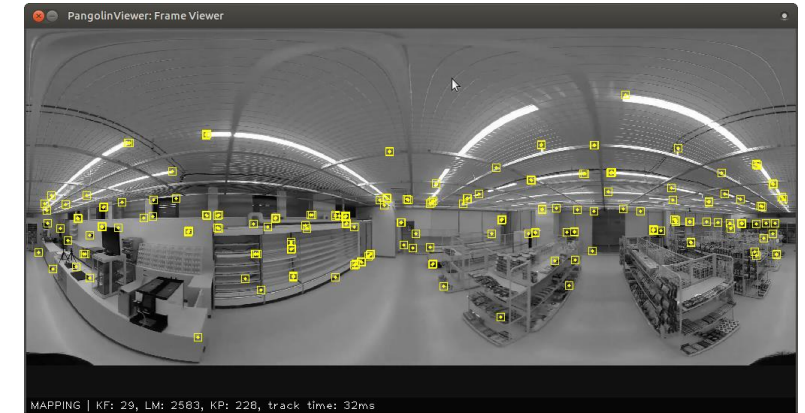
VSLAM view using a fisheye lens. Dots indicate feature extraction (to create a point cloud)
